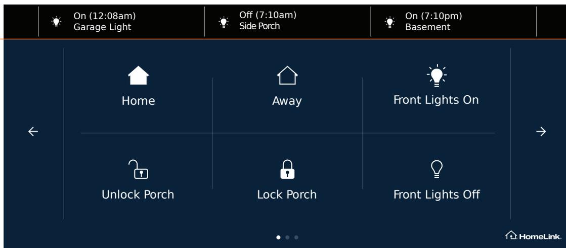
The InControl display has two separate configurable areas: Status and Buttons. Use the tabs in the app to select Status Bar or Buttons.
